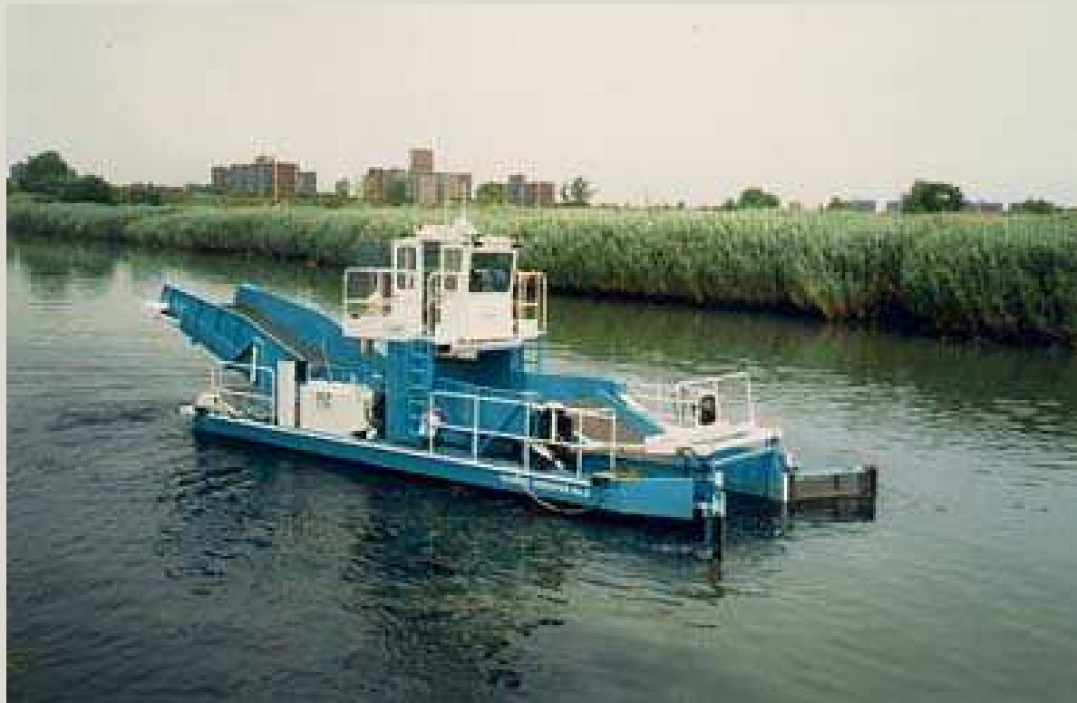
UMI TrashCat™ skimming back bay wetland areas of New York City's Jamaica Bay
