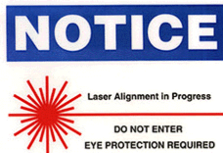
Door sign to indicate laser alignment/maintenance.
